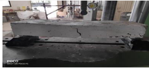
Fig 5: After 28days testing on three point loading
