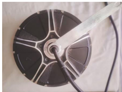
Figure 4 BLDC hub motor
