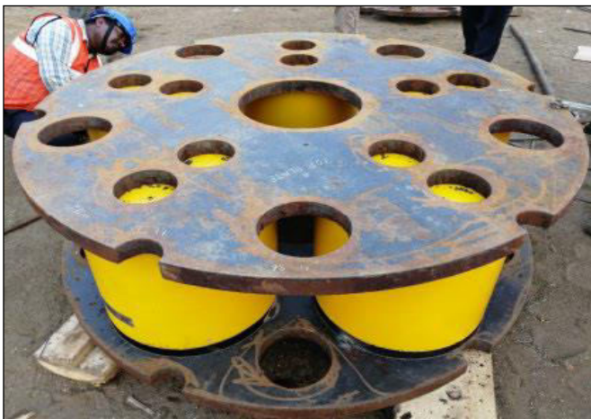
Typical details of O cell arrangement
