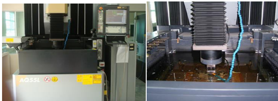
(a) Photograph of EDM during machining (b) EDM tank and sample at operational condition.
