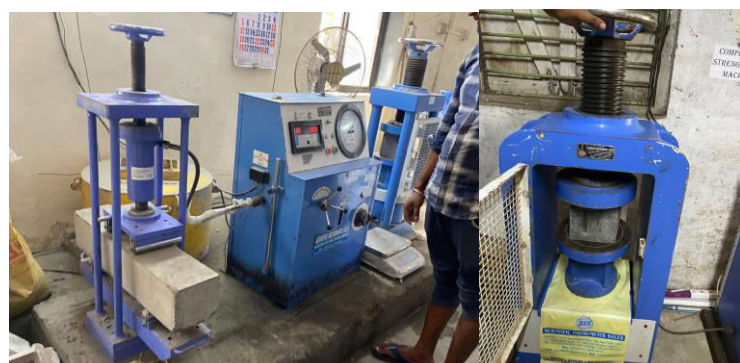
Fig 2: Flexural strength test and compressive strength test
