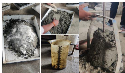
Fig 1 Concrete Mixing and slump
