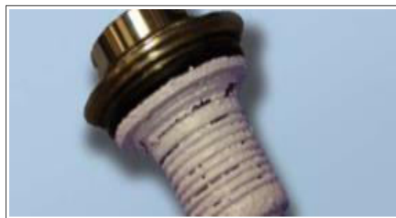
Figure 41: Mechanical Seal Spring with Solidify Fats
