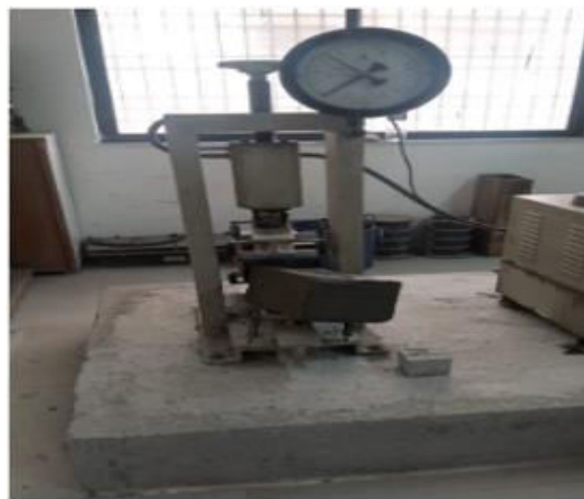
Fig 6 Flexural Testing Machine
