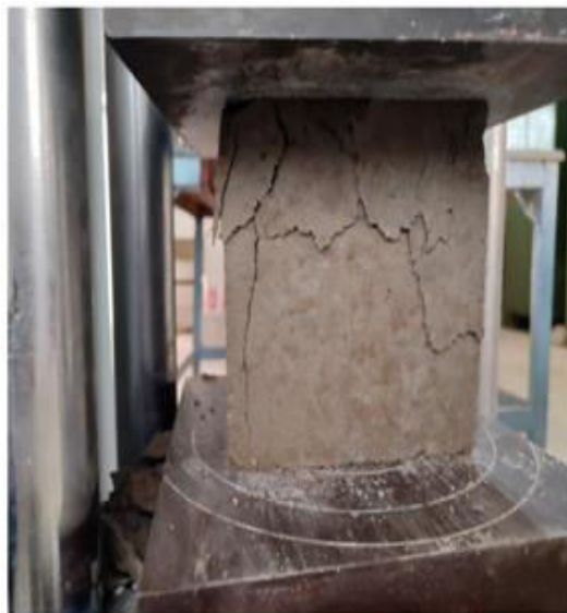
Fig 5 Testing Cube on CTM
