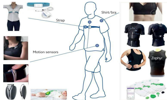
Figure 4: Location on the body of several commercially available wearable devices able to estimate ventilation from chest and movement of thoracic region.
