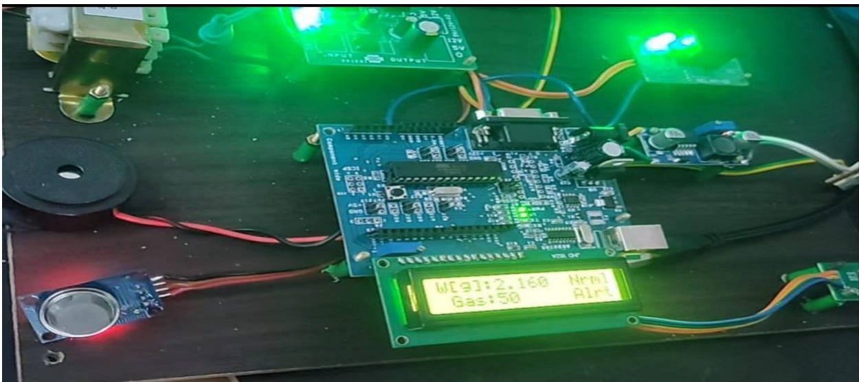
Fig 1.8 : LPG gas leakage detected
