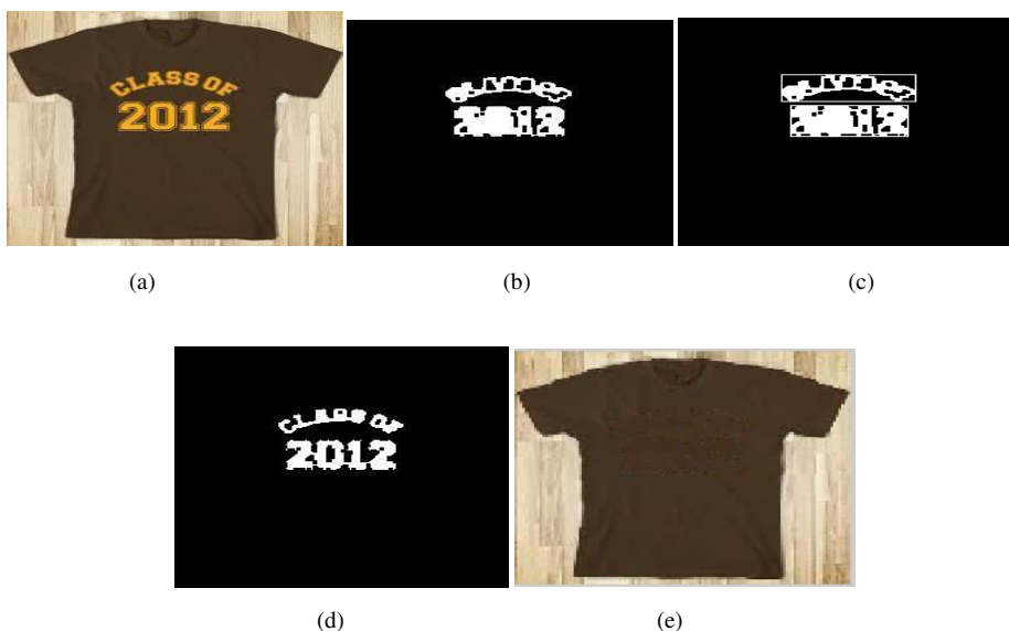
Fig. 4 Text Detection and Inpainting (a) Original image (b) image after applying first set of criteria (c) image after applying second set of criteria (d) Image mask (e) Inpainted image using patch size 5 x 5 and search window size 81 x 81
