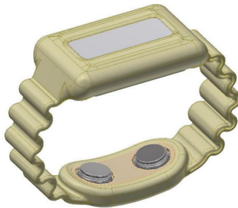
Figure 5.1 Wristband model containing electronic components and electrode device.
