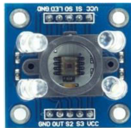
Fig [8]: Colour sensor TCS3200
