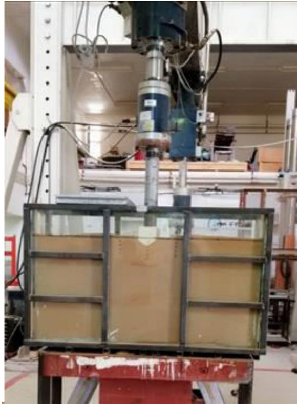
Figure 2. Experimental setup showing test tank with compacted sand
