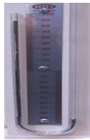
Figure 1. Photographic View of Differential Manometer
