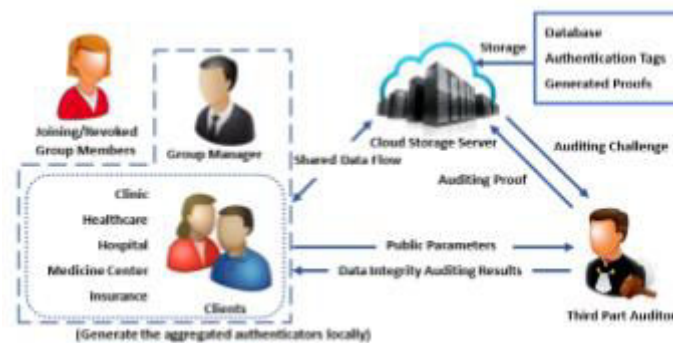
Fig. 1. The cloud storage model of our VDBscheme, which includes three entities, the cloud storage server, the clients and a Third Part Auditor (TPA)
