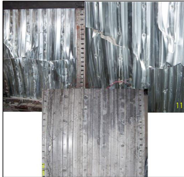
Fig. 7. Failure mode of steel sheet and concrete core under cyclic loading.
