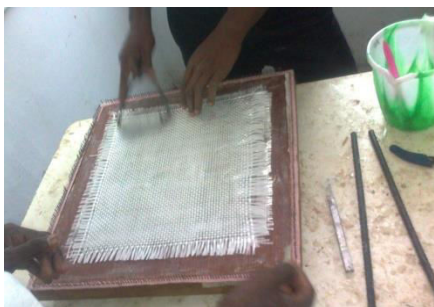
Preparation of hand lay-up process
