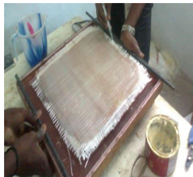
Preparation of reinforcement
