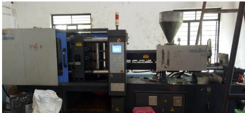
Figure 3.1 Photographic view of Milacron 110 Injection Molding Machine
