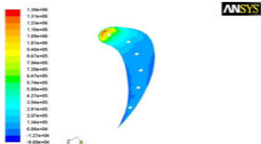
Fig4.5 Variation of static pressure of 6 holes Titanium alloy in Gas Turbine Blade
