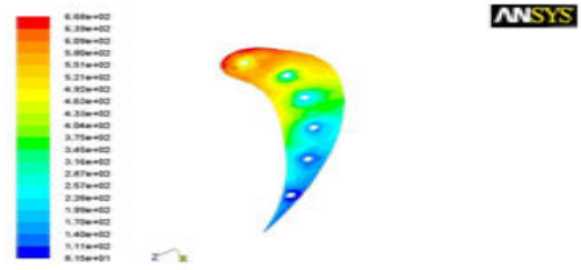
Fig4.7 Variation of static Temperature of 6 Holes Titanium alloy in Gas Turbine Blade
