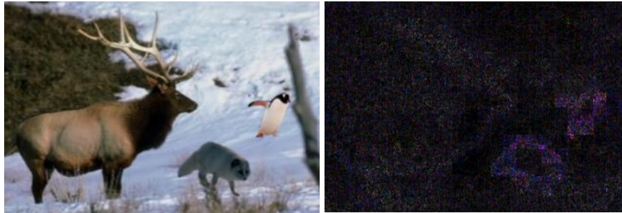
Fig 4: Fake Image and Corresponding ELA image where the spliced portions are highlighted
