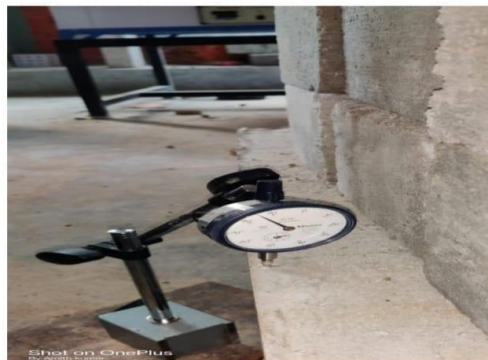
Figure 1 Strain gauge used for record the deflection
