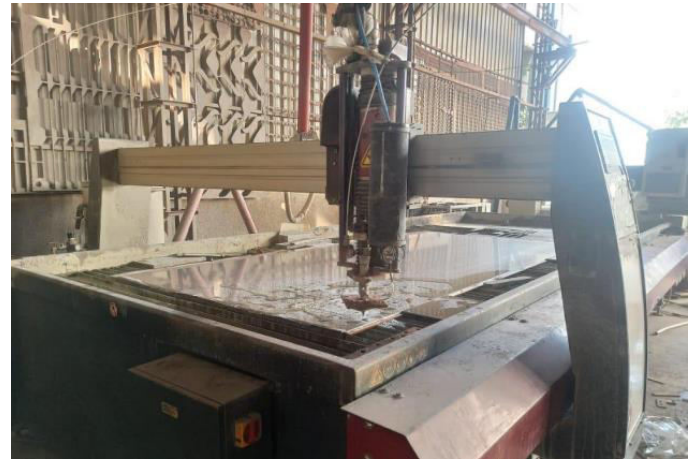
Fig. 2 : MAXIEM 2040 Jet Machining Fig. 3: Abrasive Water Jet Machining
