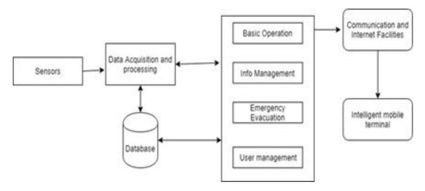
The block diagram of the system, where the current position of the evacuee will be tracked using indoor positioning with the help of a WIFI signal and leads to the short and safe exit.
