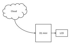
D1 mini which placed at the receiver side fetched the data stored in cloud and display on LCD. The main work of receiver is divided as follows:
