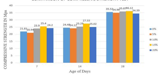
The above graph indicates that the compressive strength for 7, 14 and 28 days with 5%, 10%, 15%,20% of Waste Paper Pulp ash and Sawdust of the weight of cement. The optimum value is obtained at 15% replacement of Waste Paper Pulp ash and sawdust in compressive strength test.
