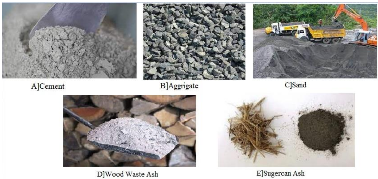
Figure No. 4 (a),(b),(c),(d) &(e) Ingredients use in concrete
