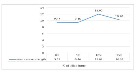
Due to the pozzolanic activity of silica fume and the filler effect, the silica fume combination was more robust thanother mixtures. The medium size of the aggregate and silica fume mixture significantly enhanced both permeability and compressive strength.
