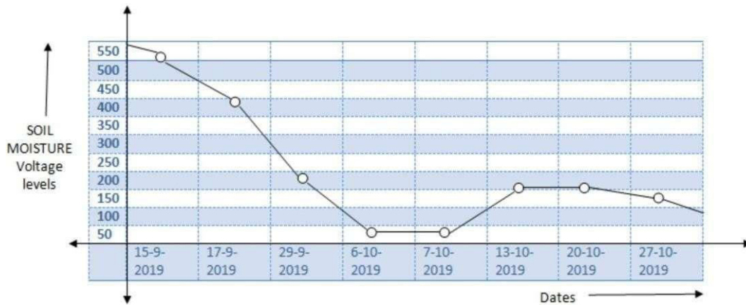
Fig. 4. Continuous manual measurement plot of the output of the sensor
