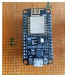
Fig. (a) ESP8266 WIFI Controller
