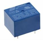
A relay is an electrical switch that operates using an electrical signal. It consists of input terminals to receive control signals and output terminals for operating contacts. The switch can have various contact forms, including make contacts, break contacts, or a combination of both.
