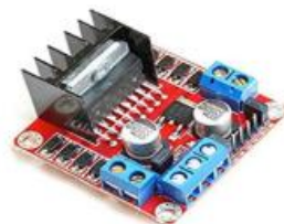
Fig 3.3 L298N Motor Driver
