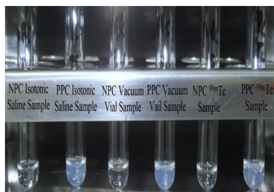
Figure 10: Negative Product Control and Positive Control for different samples. Micro tubes are kept in a dry heat bath maintained at 37 degrees ± 1 degrees for incubation for 1 hour, to obtain results.
