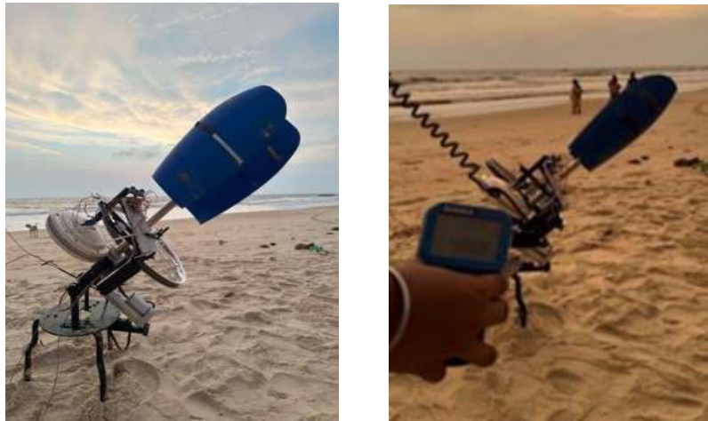
Figure 4.1.: Turbine Testing at various orientations
