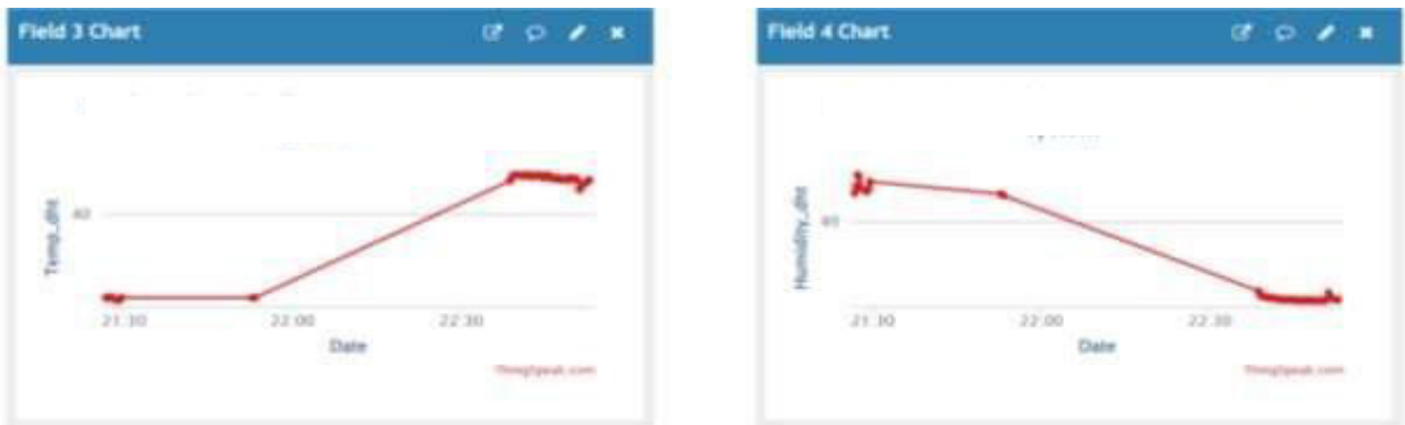
Figure 4.4 Outputs from DHT22 in ThingSpeak
