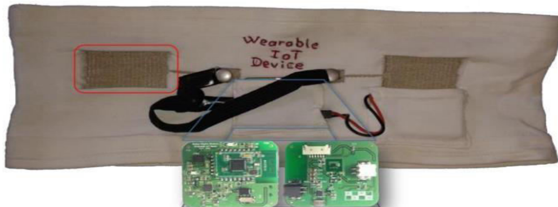
Wearable IoT Device: Illustration of the chest belt with the textile electrodes for the heart rate acquisition (red rectangle); and an inset of developed hardware for the acquisition of the parameters (front and back)
