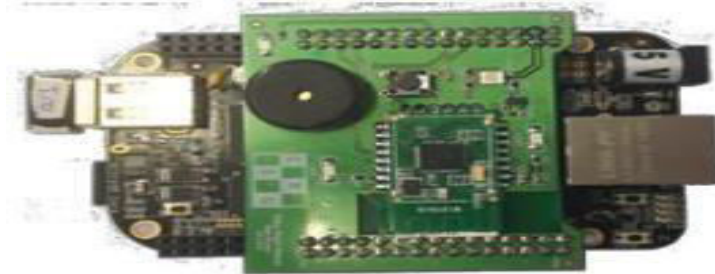
Gateway: shield placement on the BeagleBone Black
