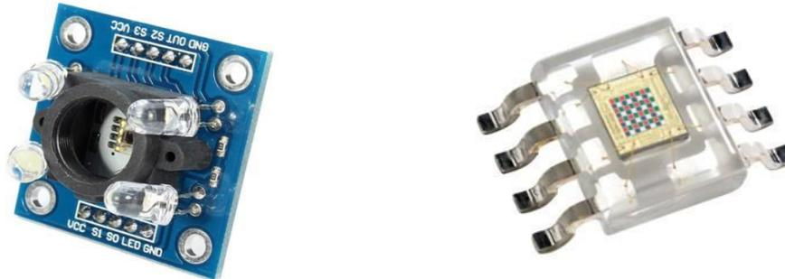
Figure 1. Photo images of (a) TCS3200 Colour Sensors (b) RGB Colour chip
