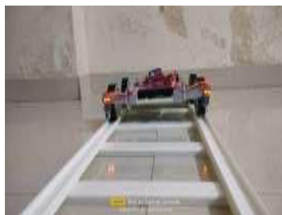
Fig. III Model of Track Fault Detector
