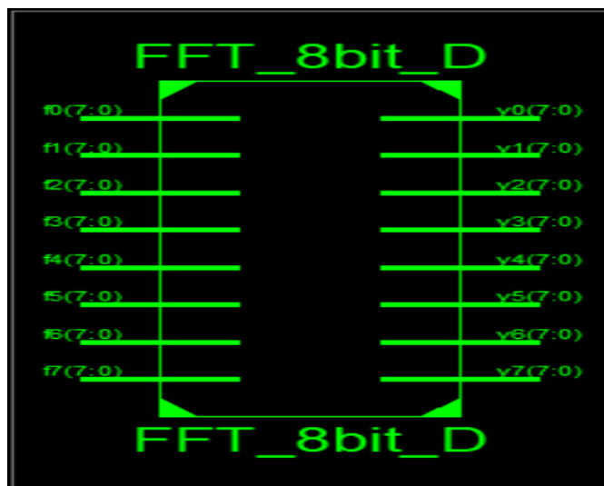
Figure 9: View Technology Schematic of 8-point DIT-FFT algorithm
