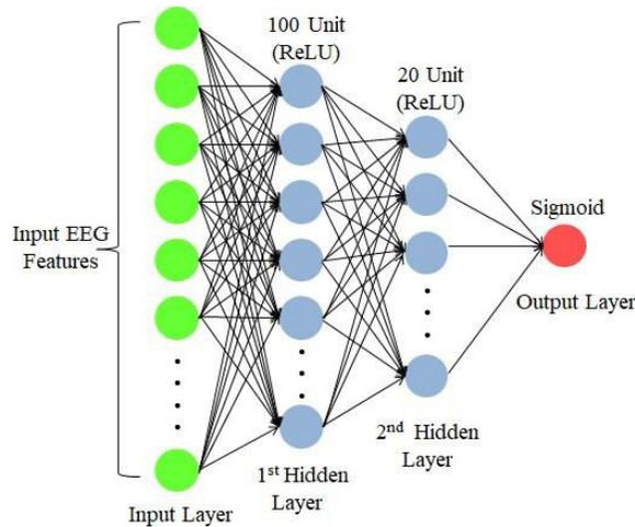
The architecture of Multilayer Perceptron Fig.
