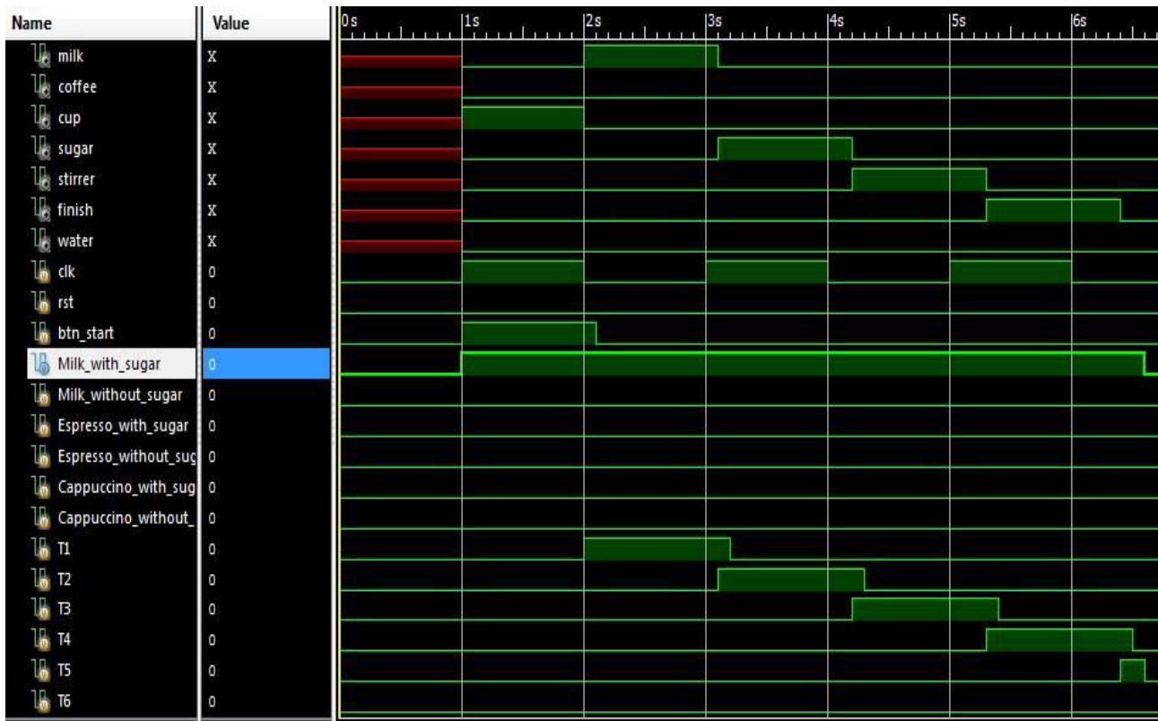
Fig. 4. Simulation results in mode of “Milk with sugar”.
