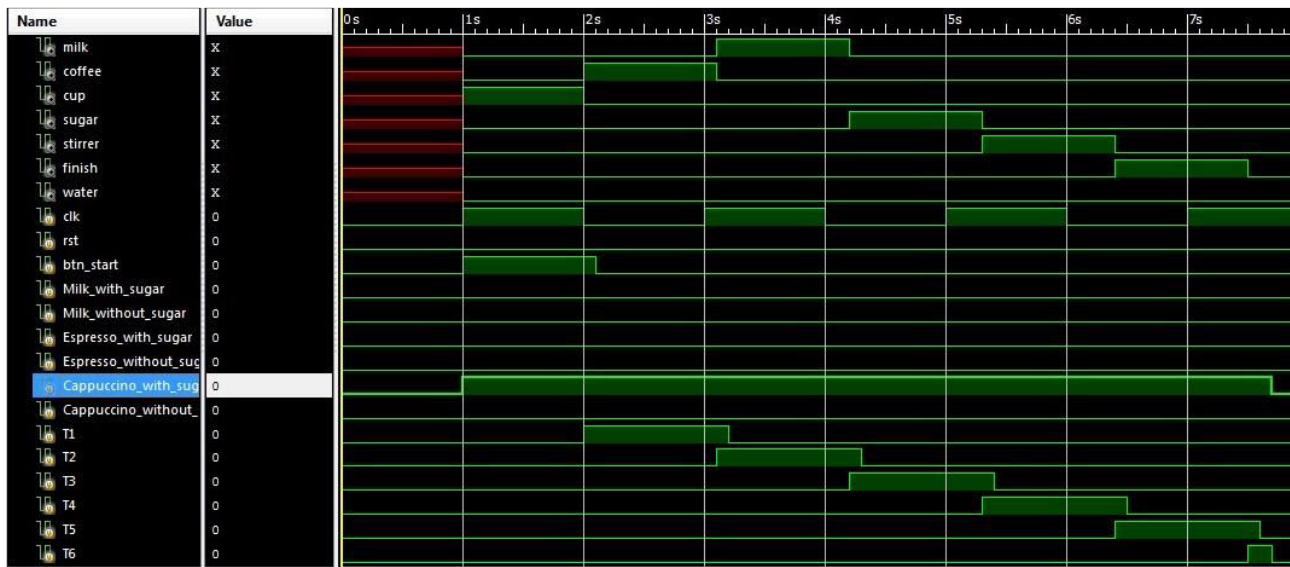
Fig. 6. Results in mode of “Cappuccino with sugar”.
