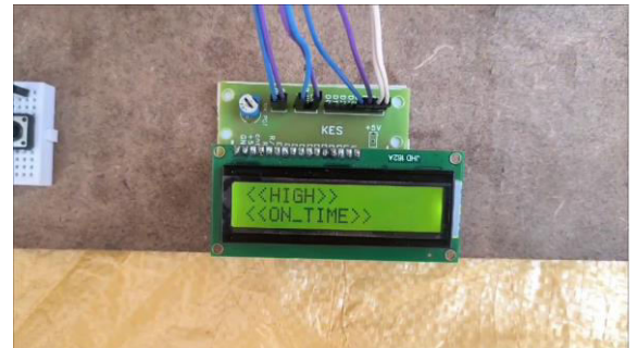
Figure 11:- Transmitter On High Speed Mode
