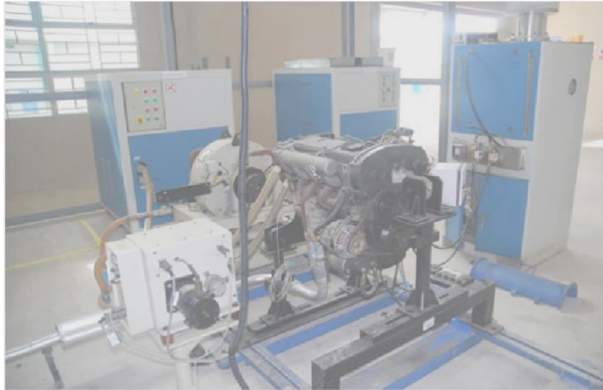
Figure 1: Mitsubishi 4D68 SOHC 2.0 L Diesel Engine Testing rig
