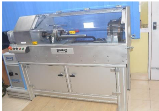
Fig5: Schatz Torque Tension Testing Machine.
