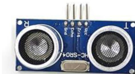
Fig 4 Ultrasonic Sensor
