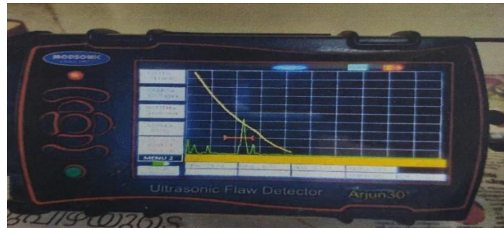
Fig 4.3 A Schematic Diagram Showing Echo Pattern. (The red line represents the DAC line any echo signal exceeding this line indicates a rejectable defect.)
