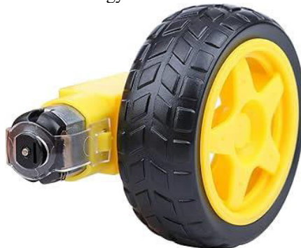
Fig 3.2.5. DC Motor with Wheel
