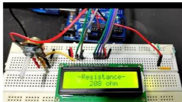
(c) Resistance 208 ohms vs Impedance 200 ohms
