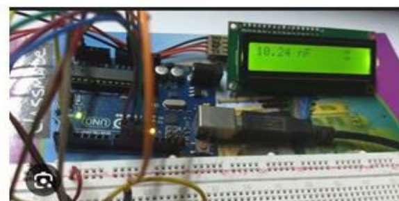
(b) Capacitor 10 nano farad
