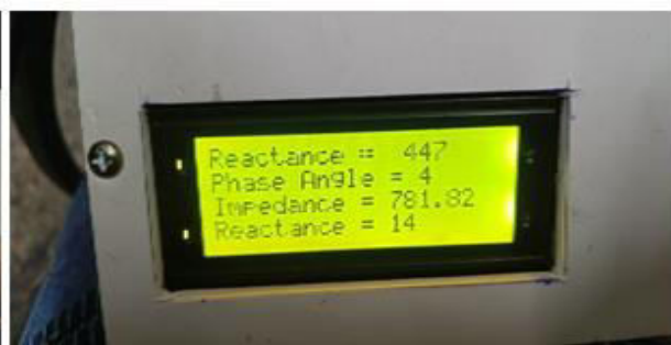
(b) Resistance 790 ohms vs Impedance 781.82 ohms
