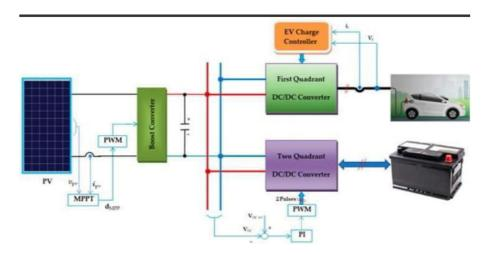
Standalone PV charging system: In off grid station, energy is provided to EV's batteries without any connection of grid [Bagher et al., 2015]. The charging system is connected with an Energy Storage Device unit (ESD) for to deliver power continuously to the EV battery during night period [Chen et al., 2016].
