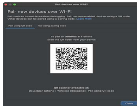
Fig 2: Popup window to pair devices using QR code or pairing code
