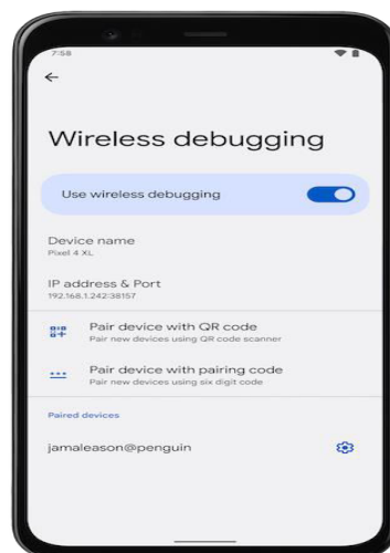
Fig 3. Wireless debugging setting on a Android phone.
