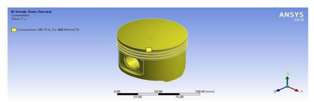
Convection is given at the remaining faces of piston to study the heat transfer characteristics
