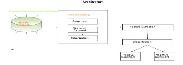
Fig: Proposed System Architecture
